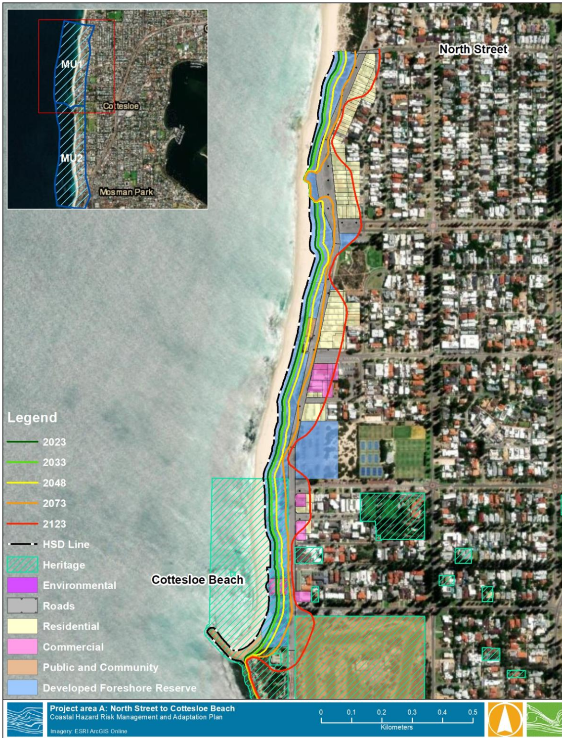
Figure 3-1 Erosion hazard lines for MU1.
