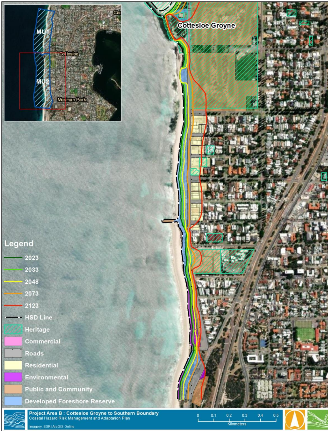
Figure 3-2 Erosion hazard lines for MU2
