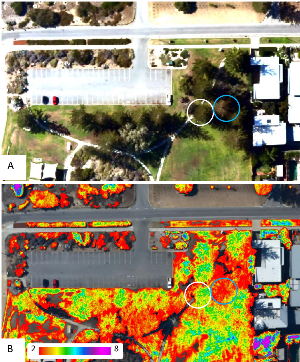
Figure 10: Difference in condition of Norfolk Island Pines in Grant Marine Park in Cottesloe. A) RGB imagery showing two Norfolk Island Pines circled in white and blue. B) The corresponding overlaid VCI illustrates the difference in vigour between the trees; the tree circled in white appears healthier and has a higher VCI compared to the less healthy tree circled in blue, which has a lower VCI.
