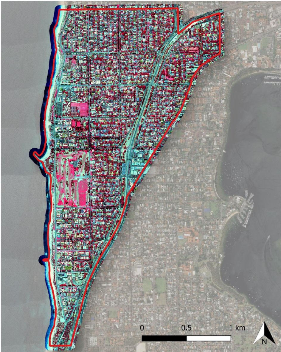
Figure 3: False colour composite over the Town of Cottesloe showing vegetation (red pixels).
