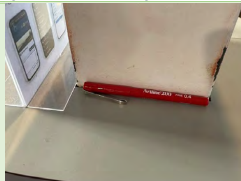
Figure 26: Minor surface corrosion
