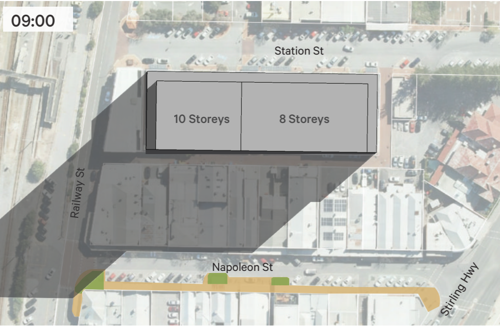
Concept B - 8 Storeys with additional 2 storeys setback from the east - 1 metre rear setback to De-Nardi Lane - 4 metre front and side tower setbacks - 56 metre eastern side setback for levels above 8 storeys
