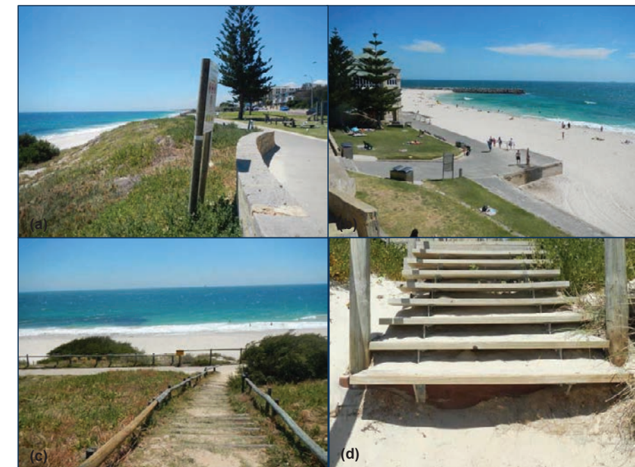
Figure 3-3 Infrastructure at Cottesloe Beach (a) majority of infrastructure/public amenity atop primary dune system (b) sea wall/amphitheatre extended to beach face (c) beach access paths both paved (background) and wooden (foreground) (d) undercutting of sediment under staircase to beach
