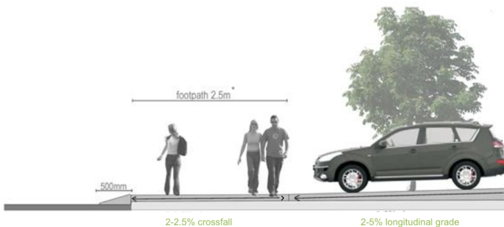
Figure 8 Typical Longitudinal Driveway and Verge Section Design
