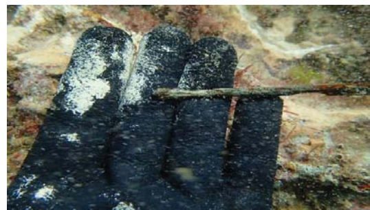
Figure 2-20 Broken ring cylindrical section
