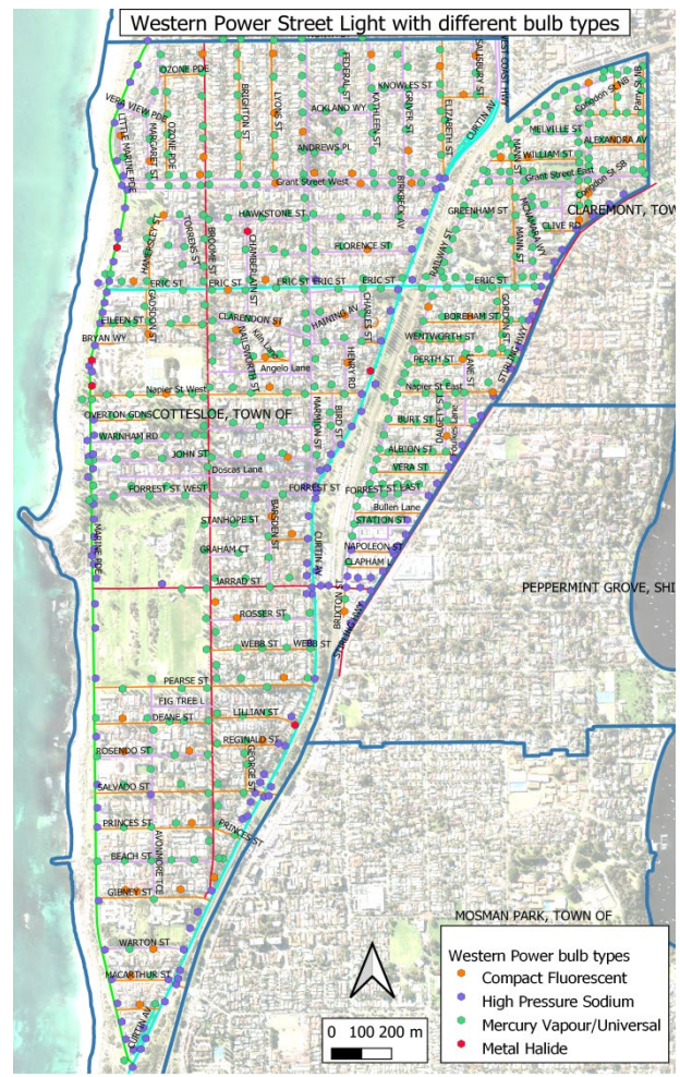
Fig 2b: Existing Western Power owned different types of bulbs within Cottesloe (data 2017).
