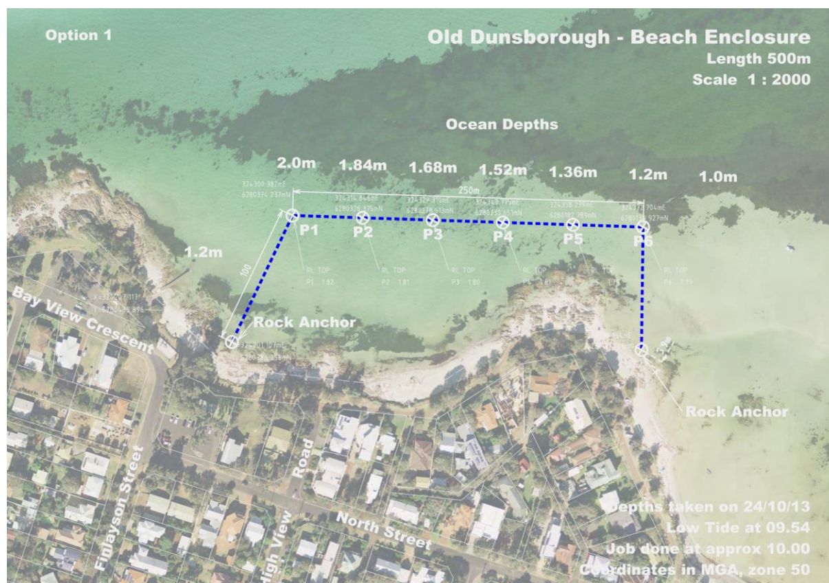
Figure 2-1 Design and layout of Dunsborough beach enclosure
