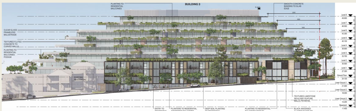
Above: Building 3 intrudes into the required 16m setback from Marine Parade above the podium level
