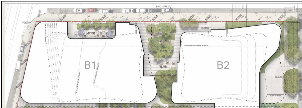
Above: Extract from proposed site plan showing reduced upper floor street setbacks to Eric Street
