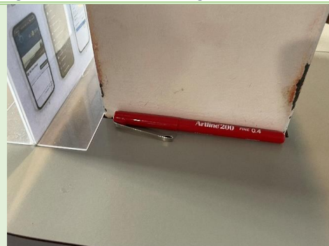
Figure 26: Minor surface corrosion
