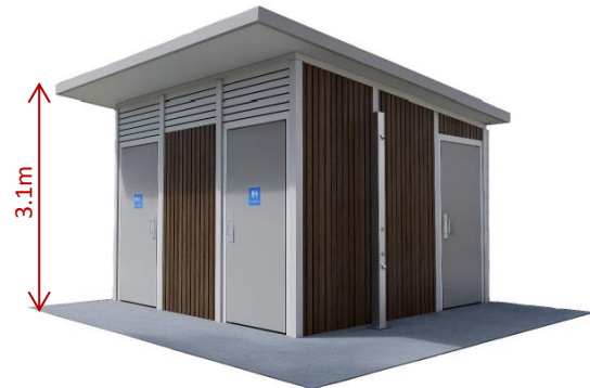
Figure 3 - Prefabricated toilet design
