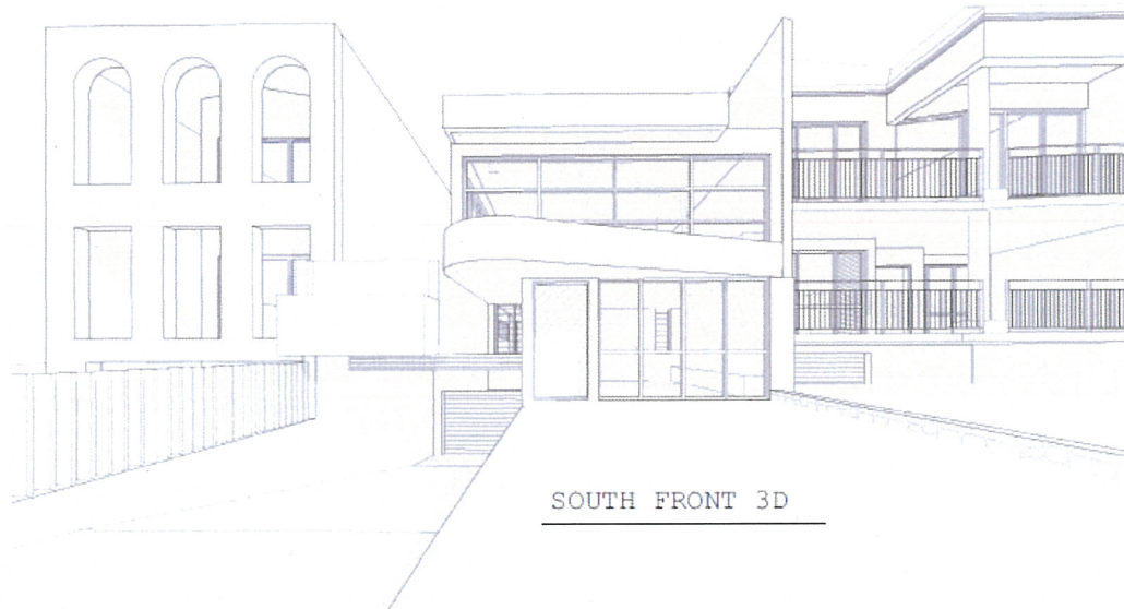
Fig. 2: 3D streetscape perspective confirming the buildings two storey appearance in relation to its neighbours. The image illustrates the skilful integration and setback of the third storey into the roof space.
