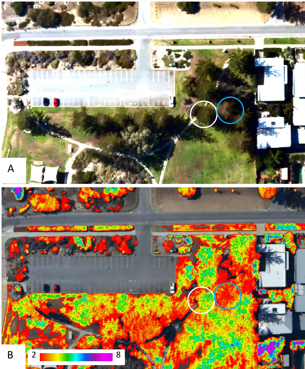
Figure 35: Difference in condition of Norfolk Island Pines in Grant Marine Park in Cottesloe. A) RGB imagery showing two Norfolk Island Pines circled in white and blue. B) The corresponding overlaid VCI illustrates the difference in vigour between the trees; the tree circled in white appears healthier and has a higher VCI compared to the less healthy tree circled in blue, which has a lower VCI.
