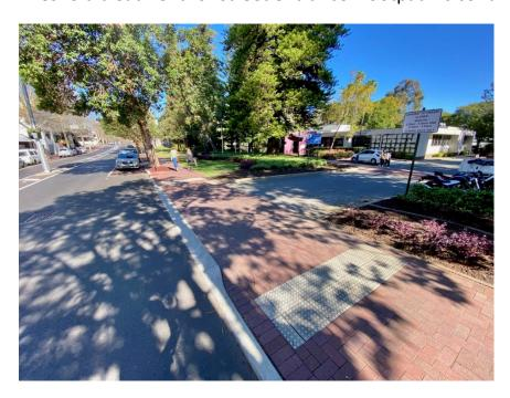
At-grade pedestrian crossing – pedestrians are prioritised with continuous grade to walk on and continuous surface, vehicles slowed by having to cross up into pedestrian space. This treatment is present at the intersection of Railway and Station Street in Cottesloe village
